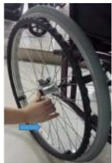
As shown in the left figure, the front wheel will be dismounted after pressing the black button in the middle of a wheel by hands, similarly, the rear wheel can be installed when the button is pressed and pushed inwards.
