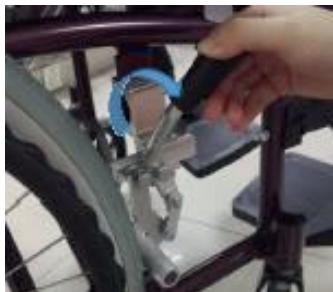
As shown in the left figure, the brake will be locked after brake hand shank is pressed forwards (the arrow direction as shown). The brake will be released after pressing operation in the reverse direction.
