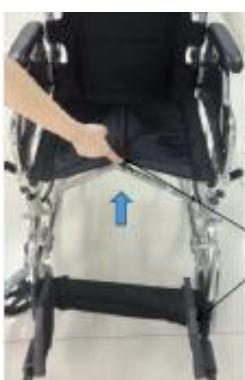
Folding: As shown in the left figure, first of all, fold the both side foot treads outwards, then, lift the middle part of the seat cushion by hands to fold the whole wheelchair.
