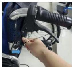
As shown in the left figure, press the button towards the outside to place the handle (as shown in the right figure).
