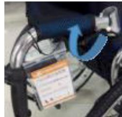
1. Hold the handrail tightly to push it towards arrow direction (as shown in the foregoing figure).
