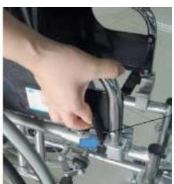
Press the button towards the body outside, then, pick up the handrail directly (as shown in the left figure).
