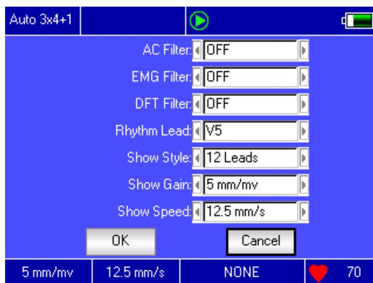
Select [OK] button and the system will apply the new settings and return to the sampling interface. Select [Cancel] and the system will return to the sampling interface without applying the new settings.
