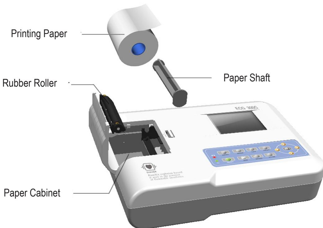
8.7.1 The dimension of the high-speed thermal printing paper in this instrument is: 80mm(W)×20m(L).
